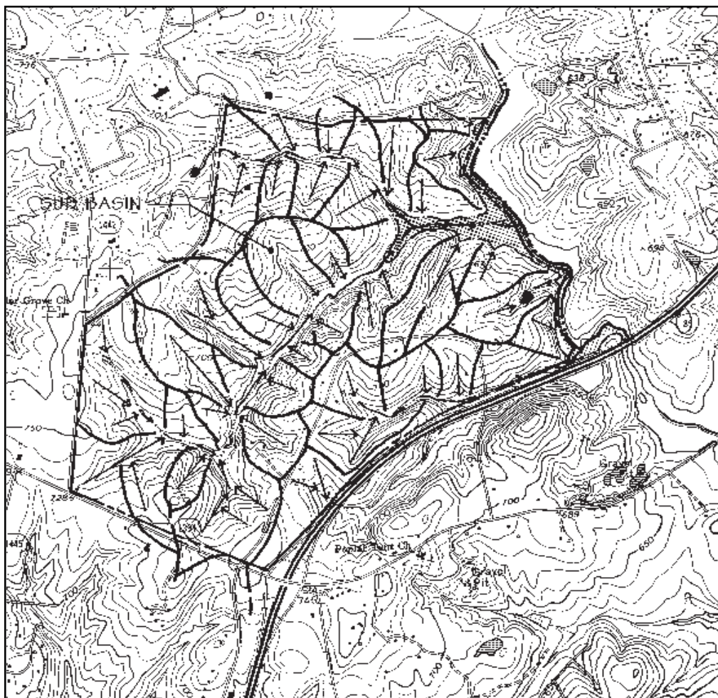
Site topography and drainage patterns can be used to divide a site into its component sub-basins for more detailed design.
